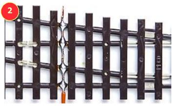
Locate the bridging point as shown above and solder this wire across all rails. We have enlarged the solder joints so you can see this more clearly. Yours would ideally be smaller blobs than this if using the right size solder.
