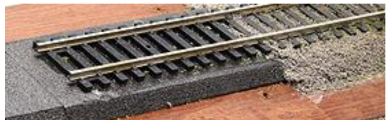
The layers - baseboard, track bed, track, ballast
