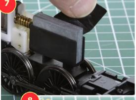
Now peel back the insulating tape that holds the additional weight into the centre of the chassis, lift out the weight and set it aside as we no longer need it (Pictures 7 and 8).
