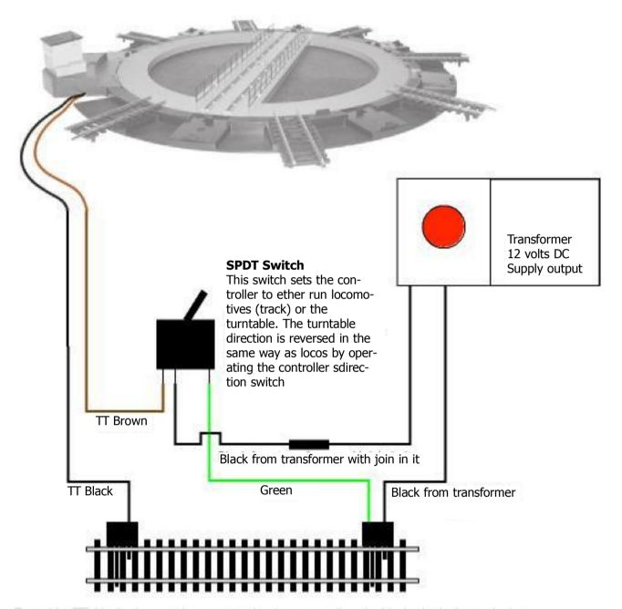
Turntable (TT) black wire must be connected to the same rail as the black wire in the track plug
